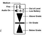
2. Press and hold the power/audio button for one second to turn off the receiver.
